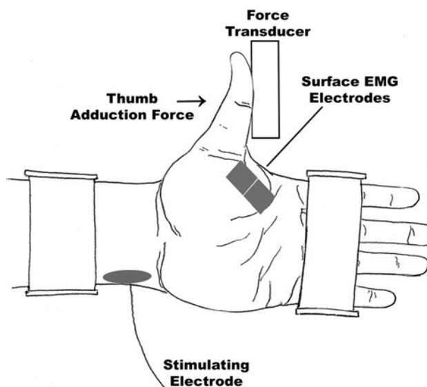
**Fig. 1** Experimental arrangement
